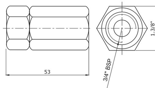
Válvula Retenção - Ref.: RTI12 (1/2" BSP) / RTI-34 (3/4" BSP)
